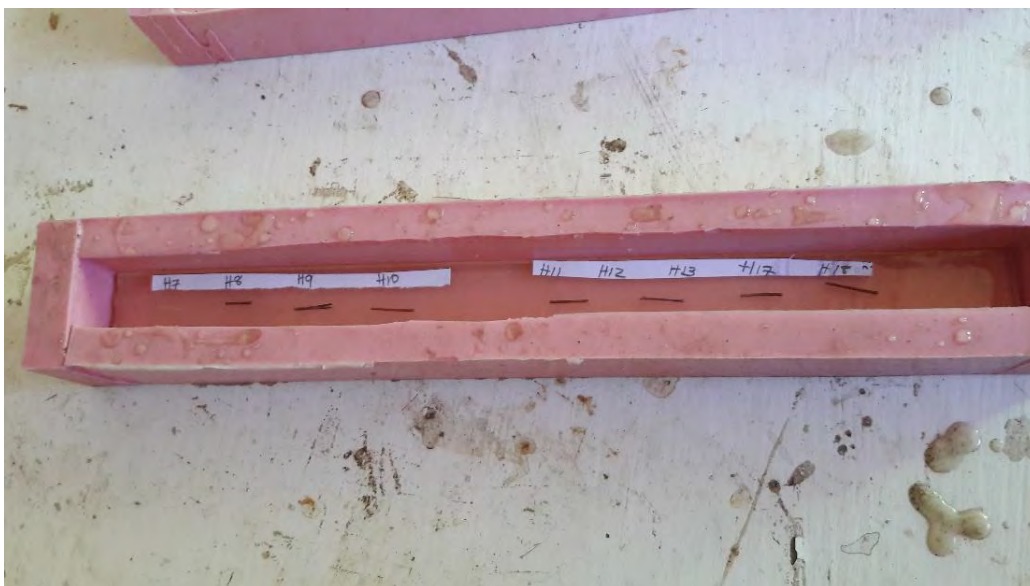
Figure 5.2: The silicon tub mould with a base layer of solidified Luxor resin, labelled paper and the 0.5 mm sectioned illicia sample of Cape monkfish, Lophius vomerinus , caught off Namibia.
