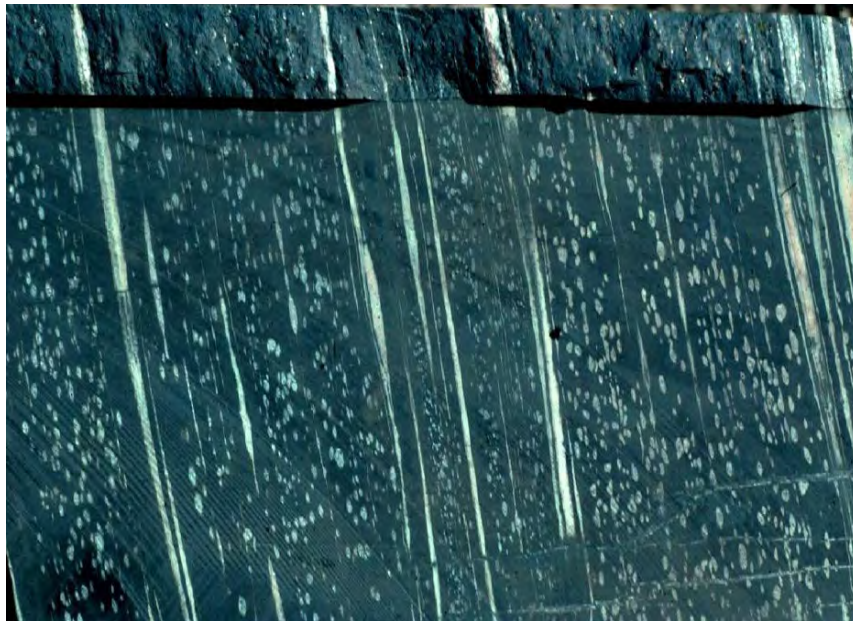
Figure 1.4. Photographic image of a halved drillcore intersection of typical Mamatwan-type, low-grade manganese ore in the Kalahari Manganese Field. Note the characteristic laminae and ovoids of Mn carbonate in a matrix of very fine-grained braunite(+hematite). Width of field of view: 8cm. (Insert reference here)
