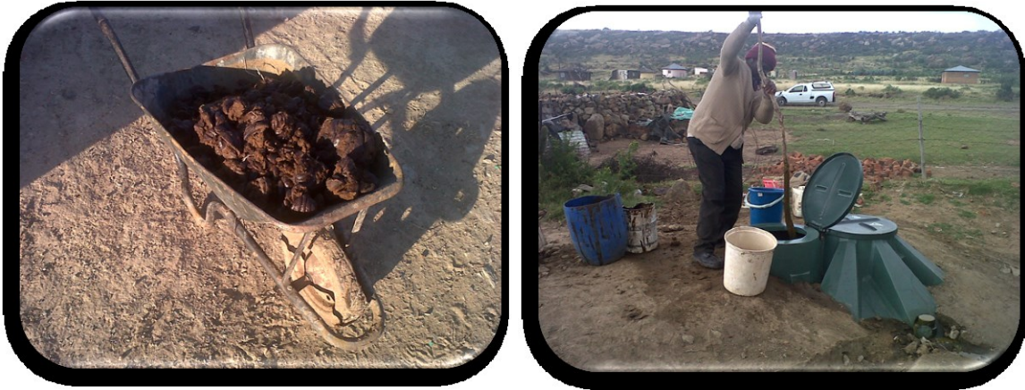
Figure 5-8: Primary feedstock is fresh cattle dung (Left). Figure 5-9: Feedstock being mixed before addition to the bio-digester (Right).
