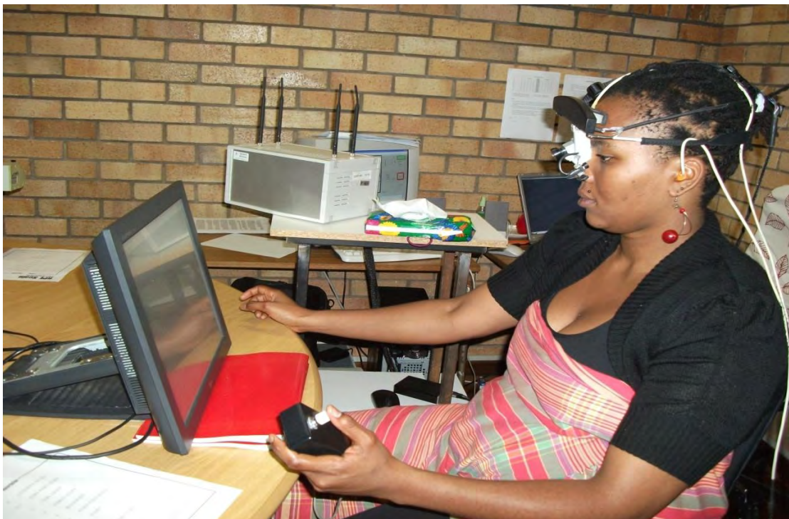
Figure 4: A participant holding the reaction time test button and conducting the Fitts task fitted with the eye tracker and temperature sensors.
