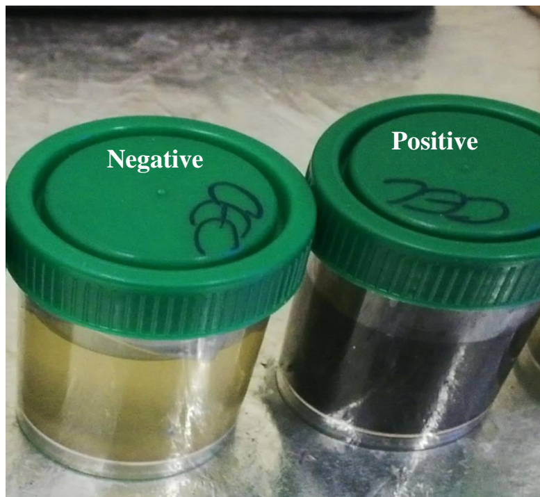
Figure 4.1: Water samples analysed by modified H 2 S kit indicating negative (left) and positive (right) results
