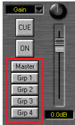
Figure A.31: Sirius Mixing Console Control Page: Group Buttons [D&R Electronica Weesp b.v., 2010b]
