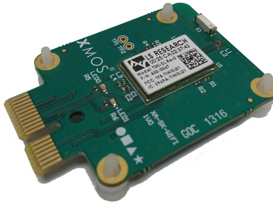
Figure 3.4: WiFi slice containing the TiWi-SL wireless module.
