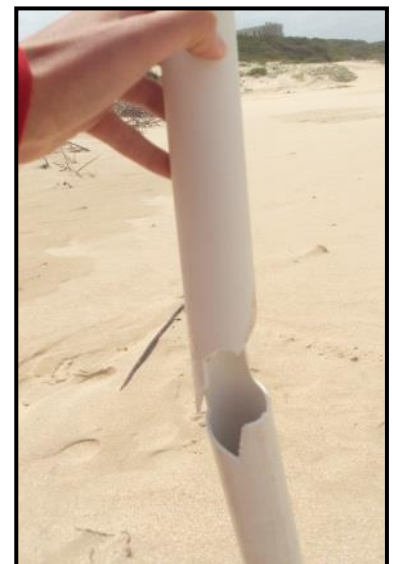
Figure 33: Broken pole from Cape St Francis wind
