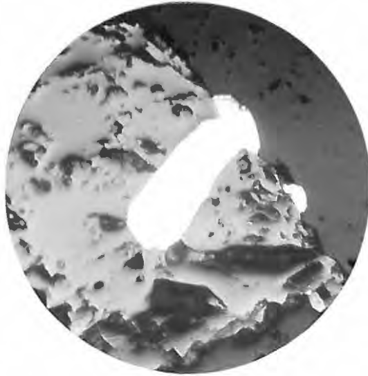
Fig.1 Coarse-grained, silver-rich gold enclosed by sphalerite. In both colour and grain size it differs markedly from gold occurring as discrete grains. x 360.
