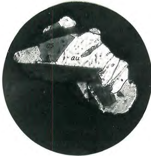
Fig.1 Intergrowth of gold (light grey) aurostibite (?) (medium grey) and tetrahedrite (stippled). The intergrowth is moulded to the faces of quartz crystals (dark grey). x 750.
