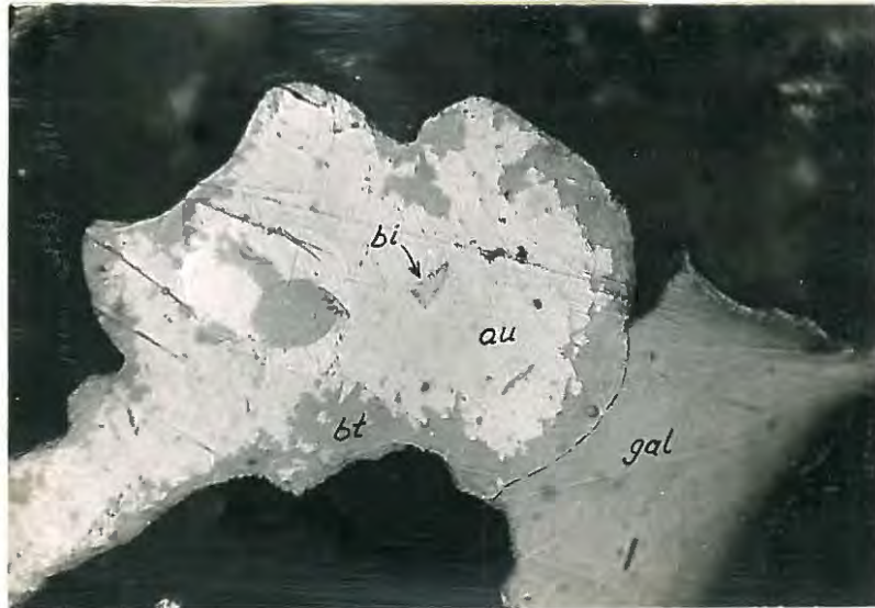
Fig.1 Gold (pale grey) partially replaced by bismuthinite (bt). The large grain on the right, indistinguishable in the photograph from bismuthinite, is galena (gal). Note native bismuth (bi) in gold. New Coburg mine. x 360.
