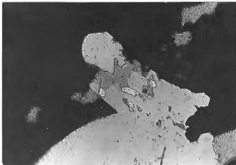
Fig.1 Pale-yellow gold (light grey) and galena (deeper grey) replacing and sending off tongues into arsenopyrite (medium grey). x 360.
