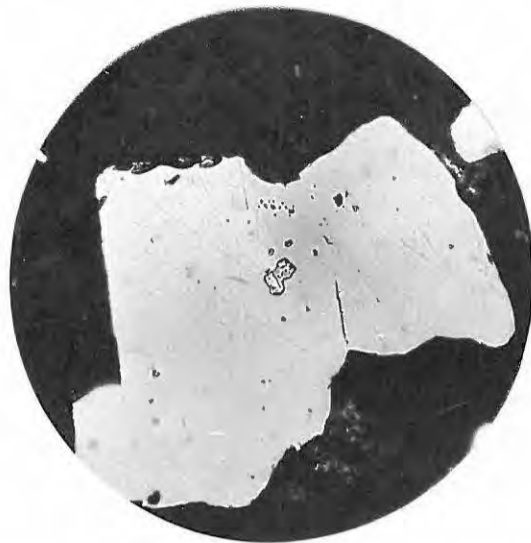
Fig.1 Gold granules (centre of field) in pyrite from Turk mine. Note larger central grain with a halo of smaller granules, a mode of occurrence which seems to be common in this ore. x 360.
