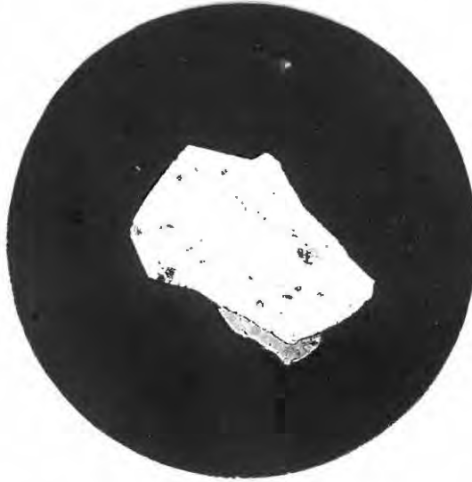
Fig.1 Gold grain partly rimmed by younger aurostibite(?) (tarnished). x 360.
