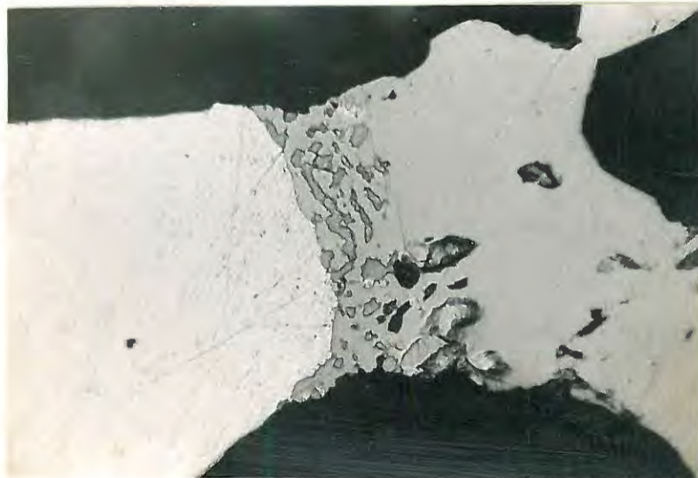
Fig.2 Aurostibite (?) (deeper grey) and tiny grains of gold (white) replacing pyrrhotite (lighter grey) in the centre of the field. Chalcopyrite is moulded on pyrrhotite on the right, and an exceptionally large grain of gold occurs on the left. Slightly etched with KOH. x 360.
