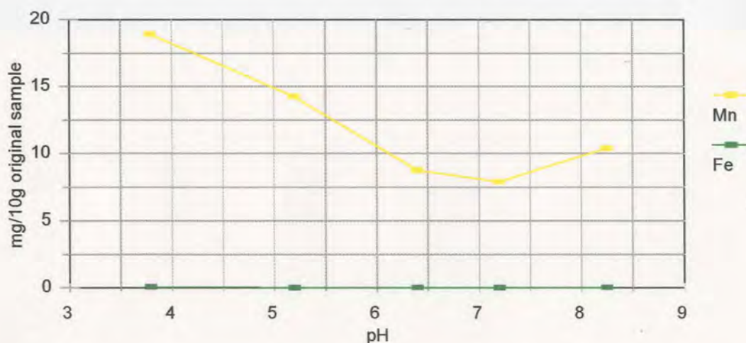
Figure 2.3 Analysis of the second filter cake after hydroxide precipitation and carbonation
