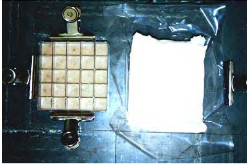
Plate 3.1 Bioassay tray (with 25 cells) filled with artificial diet, with paper towelling, plastic sheet, plastic lid (underneath) and Bulldog clips, used for closing and sealing the tray. These trays were tested and used for dose-response surface dose bioassays with CrleGV-SA against neonate and fifth instar C. leucotreta larvae.
