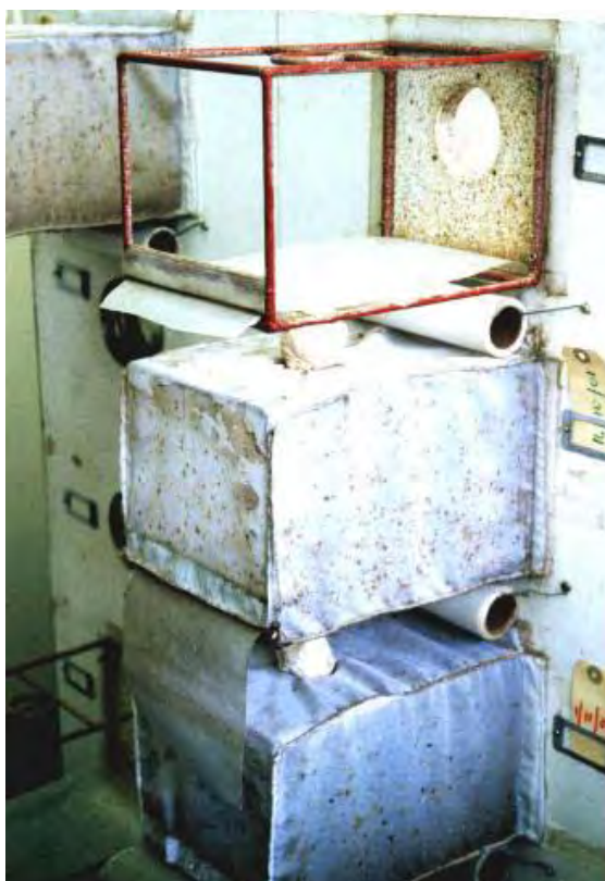
Plate 4.9 Incorporated moth eclosion and oviposition unit (Design IV) for C. leucotreta . The oviposition cage on the top right is not covered with netting so that the wax paper conveyer belt system can be demonstrated.
