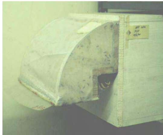
Plate 4.8 Incorporated moth eclosion and oviposition unit (Design II) for C. leucotreta moths.
