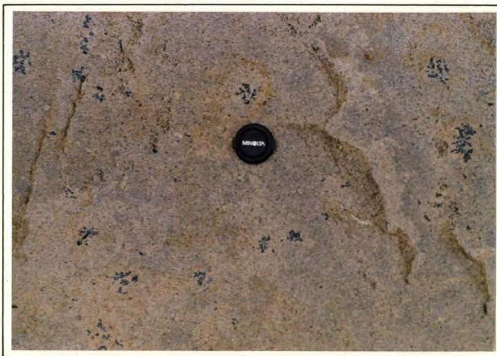
PLATE 4.20. Tourmaline nests within potassic altered Ombu granodiorite. Tourmalinization may indicate the start of greisenization.
