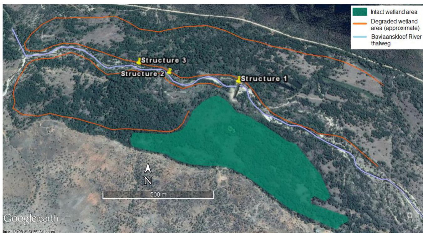
Figure 7.5: An aerial view of the location of the proposed gabion weir structures in relation to degraded and intact floodplain wetland for the proposed rehabilitation reach. Structure 1 which was built between 2014 and 2016 is visible in the google earth image, dated 2016.
