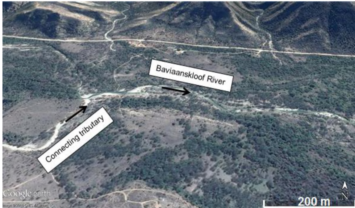
Figure 6.5: Example of a cut-and-fill river style along the middle of the study reach. The arrows indicate direction of flow of the trunk stream and a connecting major tributary.
