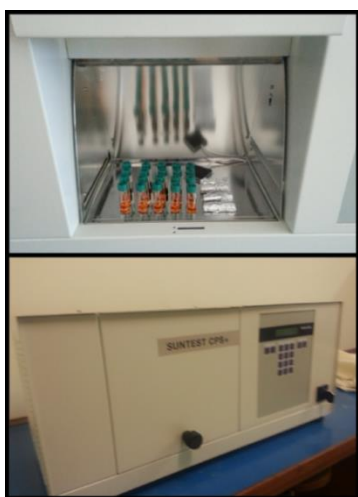
Figure 6.4: Suntest CPS+ and presentation of samples in the test chamber.
