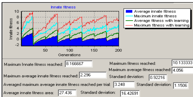
Figure 7-5 The Darwinian evolution and reinforcement learning model's innate and learning performance in an environment with fitness consequence alternations every 25 generations.
