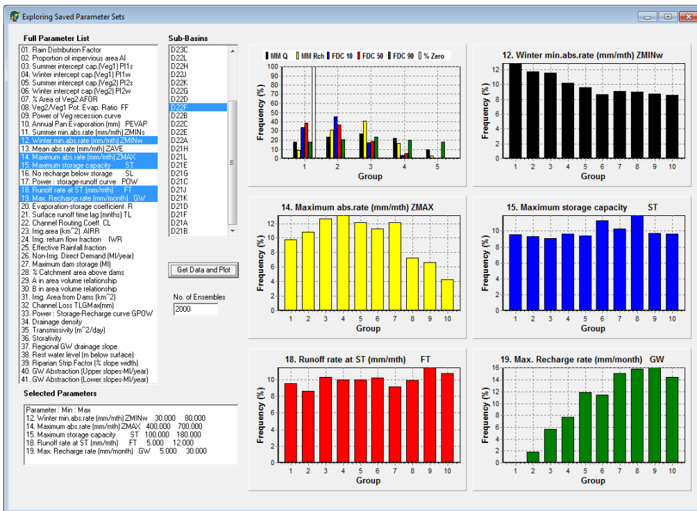
Figure 4.6 A successful sub-basin with 2 000 behavioural parameter sets generated with well distributed parameters and constraint values
