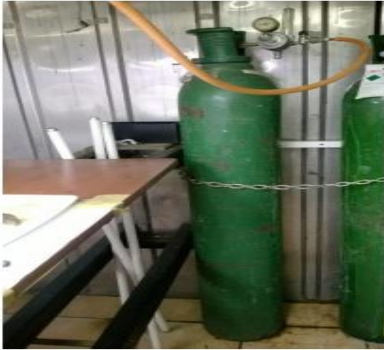
Figure 30: Compressed carbon dioxide gas cylinder connected to a carbon dioxide regulator (Mogane, 2016).
