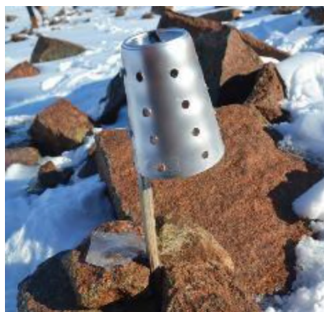
Figure 26: Radiation shield used in the field. Source: R. Dwight.
