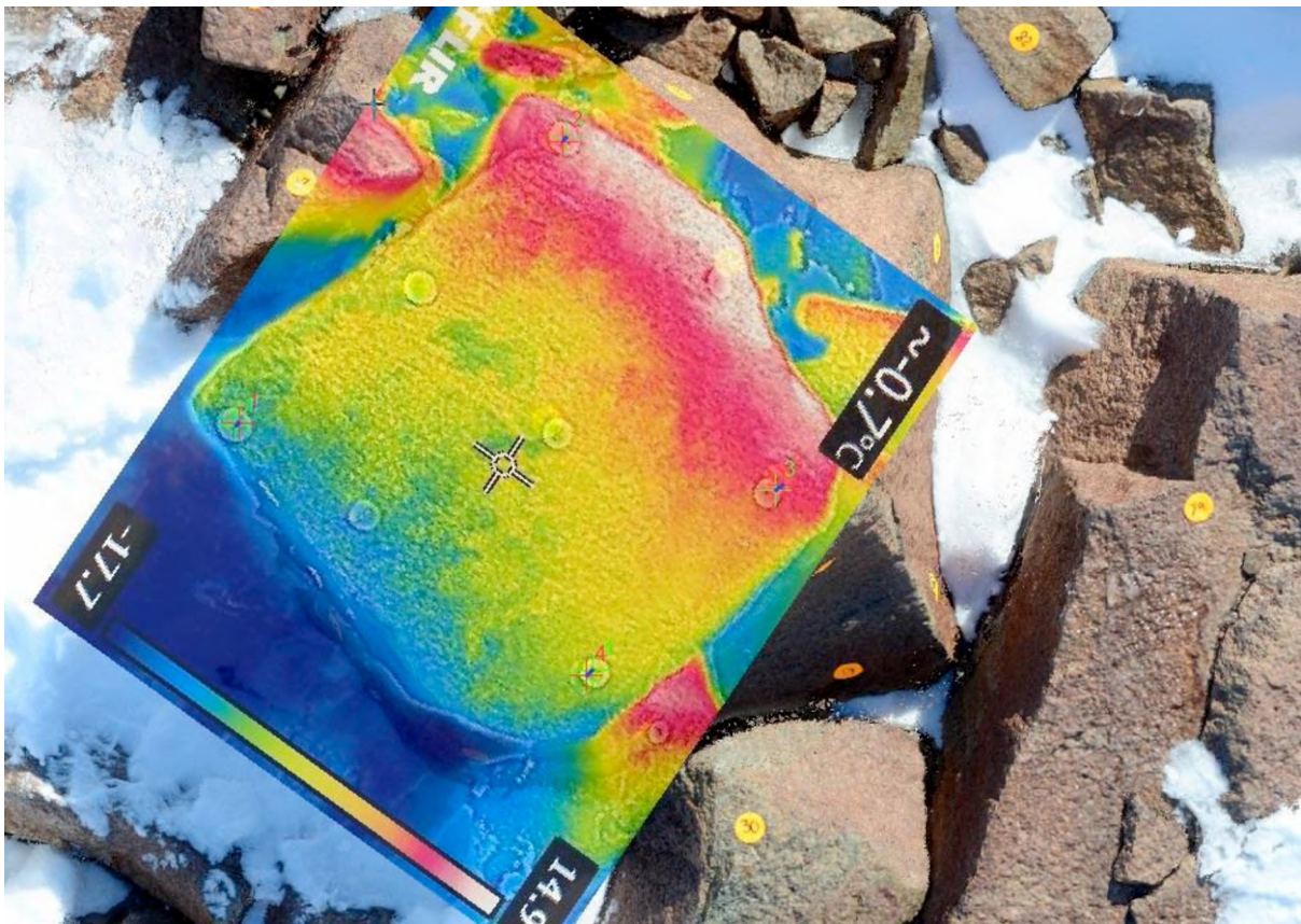
Figure 53: Georeferenced FLIR image in ArcMap®.
