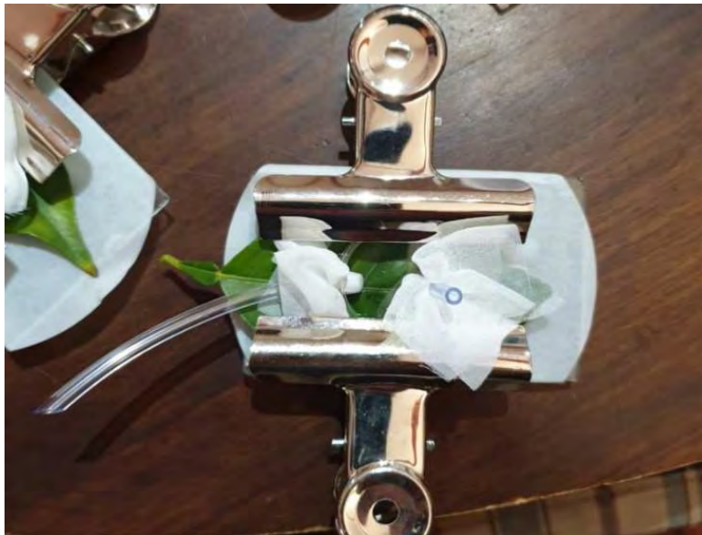
Figure 2.1 Final assembly of test cells on top of a leaf containing an aged residue of insecticide and loaded with live A. vladimiri wasps.
