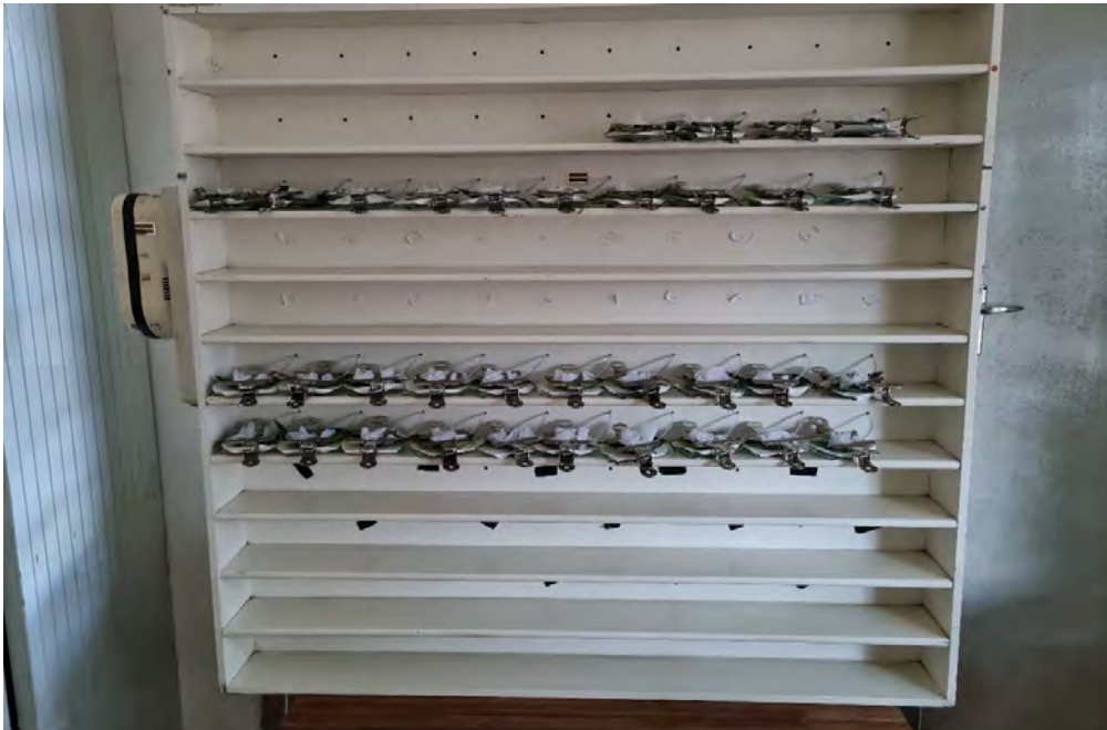
Figure 2.2 A maximum of 10 replicate test cells connected to a plenum providing a constant air flow generated by an electric fan (attached to left wall of the plenum).
