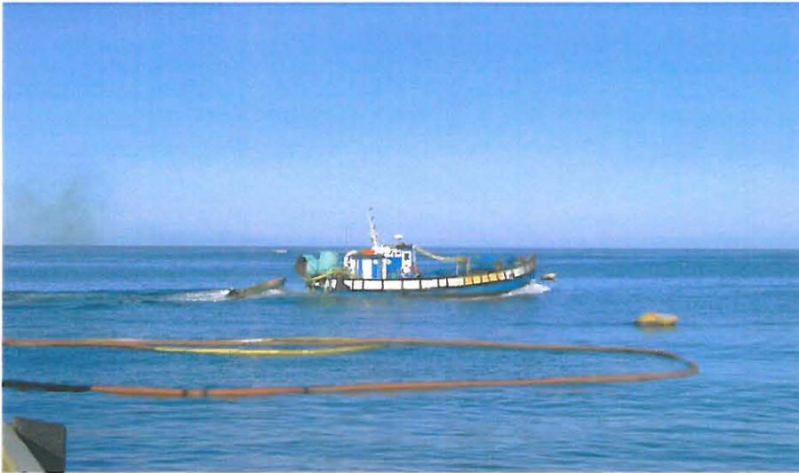
Plate 5.5: Mining diamond boats used along the Namaqualand coastline. Note the extended pipe used by the divers when operating from the boat.
