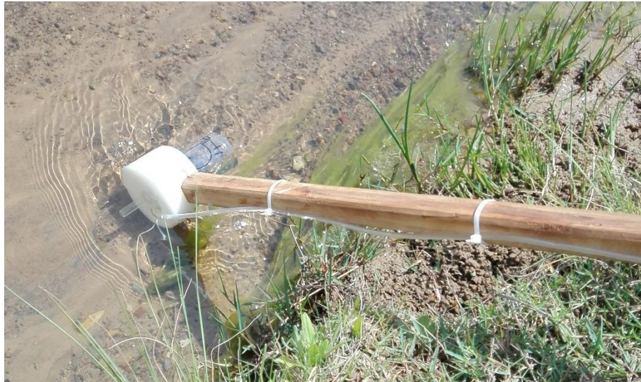
Figure 4.2: Depth-integrating sampling pole with a sample bottle attached
