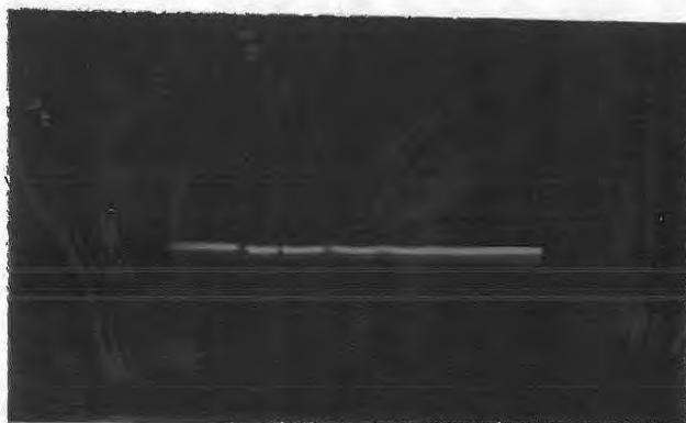
Fig. 1.20 - Effect of placing a lead sheet with slit in front of C.R.O. screen.
