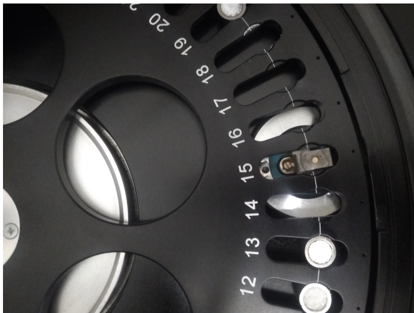
FIGURE 4.4: A picture of the heater at position 15 with the sample carousel in place.
