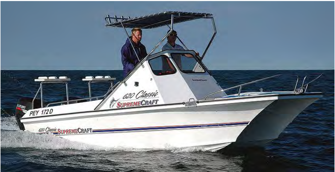
Plate 2.1a A typical catamaran-type hull ski boat powered by two large outboard engines (Photograph from www.africanangler.com ).
