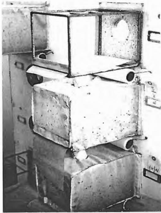
Fig 4.4 Emergence box with cages attached incorporating both oviposition and eclosion into one unit.
