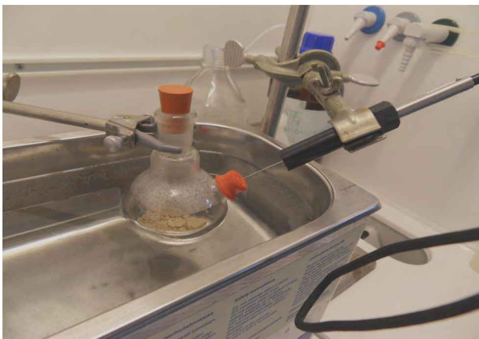
Fig. 3.4.9.1 Sampling for volatile organic compounds using SPME
