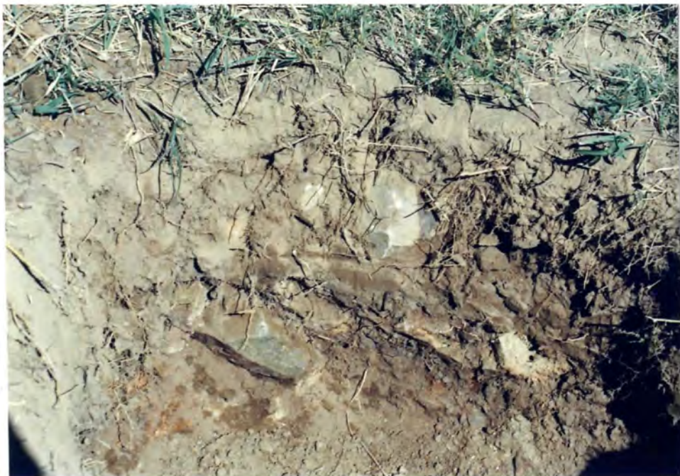
FIGURE B.2: Soil profile in the natural vegetation of the Glenrosa soil form
