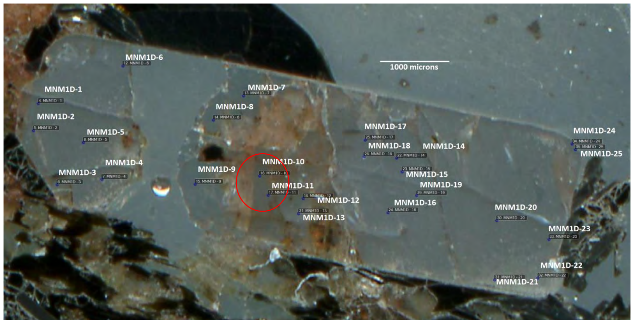
Figure 6.9B: Euhedral zircon image showing some laser-ablation pits for MNM1D. The red circle encloses two points that suggest an inherited core; more details are given in the text.
