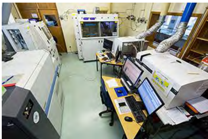
Figure 5. 4: Equipment used to analyse trace elements and REE: a Resolution 193 nm Excimer laser ablation system connected to an Agilent ICP-MS at the Central Analytical Laboratory (CAF) at Stellenbosch University in South Africa.
