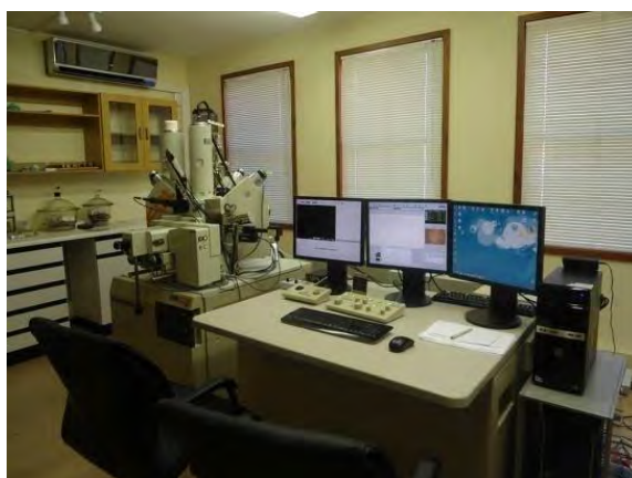
Figure 5. 2: JEOL electron microprobe at Rhodes University that was used for major and minor element analysis for mica and CL analysis.
