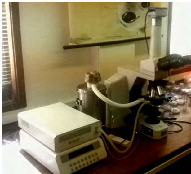
Figure 5.5: Equipment for microthermometric measurements: a calibrated LINKAM TMH 600 heating and freezing stage, together with a TMS93 temperature controller and programmer and a liquid nitrogen pump (LNP93/) cooling system mounted on Nikon Eclipse E600 transmitted-light microscope with objective lenses of 4x to 100x magnification. A DeltaPixInvenio Camera is fitted to the microscope. The equipment is housed at Rhodes University, Geology Department R.S.A.
