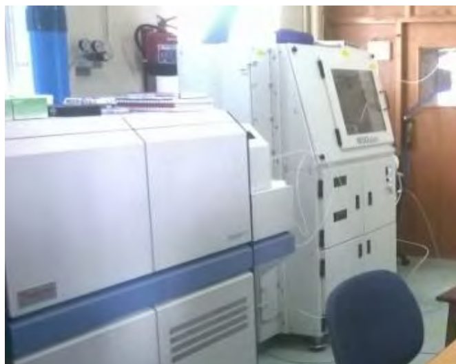
Figure 5. 1: Equipment used to analyse U-Pb isotopes: ThermoFinnigan Element2 Laser Ablation - Single collector - magnetic sectorfield - Inductively Coupled Plasma - Mass spectrometer (LA-SF-ICP-MS) at the Central Analytical Laboratory at Stellenbosch University in South Africa.
