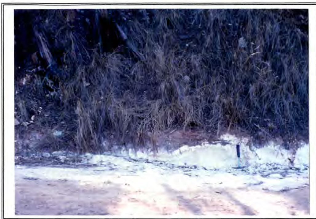
Figure 4.10 Photograph looking east showing weathered clay-sericite-quartz rock inbetween the N° 3 Leader and Main Reefs at the Harewood deposit. Quartz reef float is evident along the left-hand margins of the photograph.
