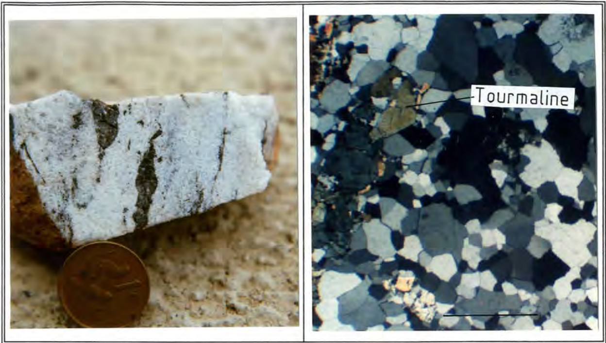
Figure 4.7a Photograph of tourmaline-bearing, auriferous, saccharoidal vein quartz from the Harewood Au working. Note the equigranular nature of the quartz grains and the characteristic pale greyish colour - a function of the tourmaline (plus specularite) content.
