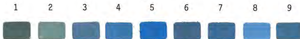
Figure 2: Colours produced after spraying spots of the various indoles with Van Urk's reagent, drying at 95°C and leaving for 24 hours. Colours vary with age and caution must be exercised when used for identification purposes. Spots from left to right-1 = serotonin, 2 = 5-methoxytryptamine, 3 = N-acetylserotonin, 4 = melatonin, 5 = 6-hydroxymelatonin, 6 = 5-hydroxyindole-3-acetic acid, 7 = 5-methoxyindole-3-acetic acid, 8 = 5-hydroxytryptophol and 9 = 5-methoxytryptophol.
