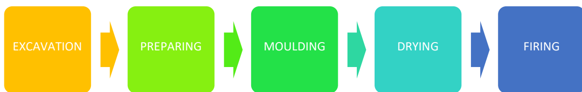
Figure 2.3: Showing the steps in the process of traditional brickmaking (adapted from Amyikaiye et al., 2021, p. 7)
