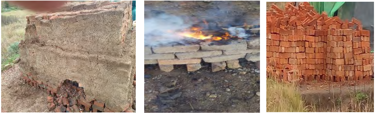
Figure 5.10: Showing the last three practical stages of the traditional brick-firing process: (d) firebox at the bottom of the clamp kiln (e) fire burning on the firebox (f) de-hacked bricks arranged
