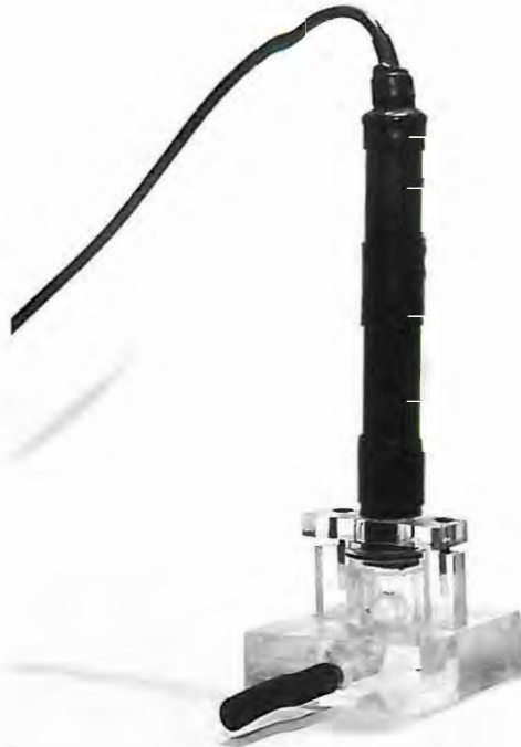
Fig. 34. The pH probe mounted in a chamber so that water flowed in the bottom around the glass bulb, and out at the top. Ducts from the top of the chamber ensured that bubbles were not trapped.
