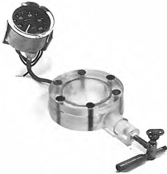
Fig. 26. Perspex pressure chamber used to subject G. lignorum to pressure.
