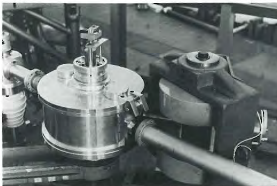
Fig. 2. A view of the target chamber and magnetic analyzer.
