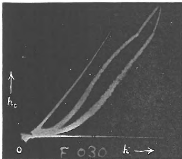
Fig. 2. Po-Be source \gamma -rays and neutrons.
