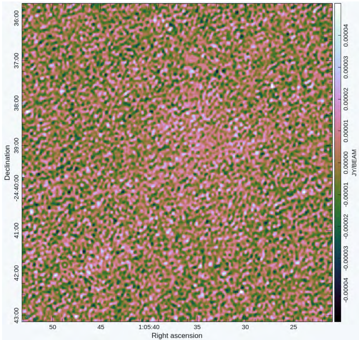
Figure 3.10: Uniform weighted residual image, zoomed at the cluster position. The noise rms is 9.0 \mu\text{Jy beam}^{-1} , and the angular resolution is 5.1'' \times 4.4'' . Compared with Figure 3.9, we can see that sources were subtracted accurately, without any apparent residual error, leaving a fairly uniform residual across the image.
