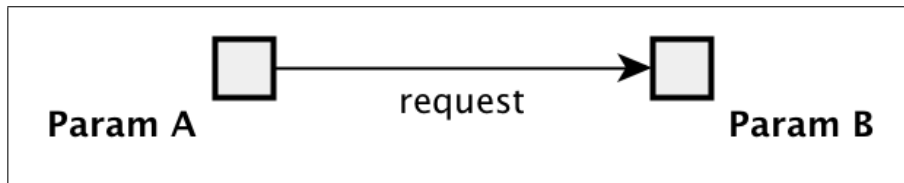
Figure A.2: An AES64 request message which does not demand a response.
