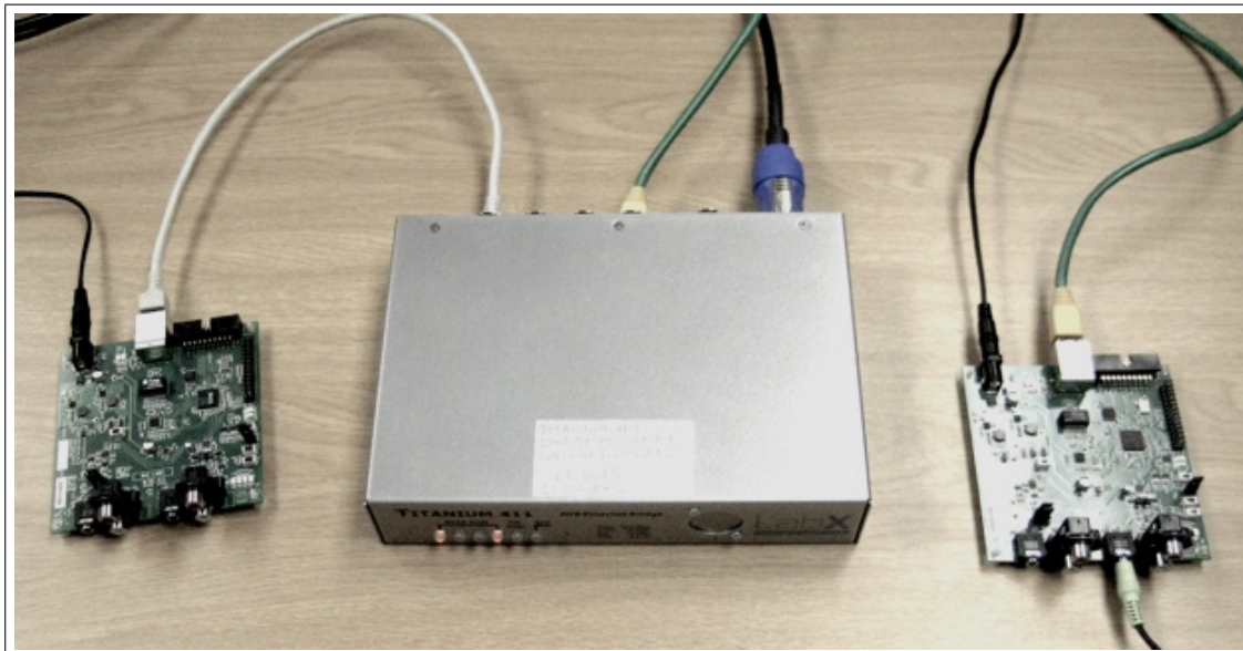
Figure 2.26: A simple AVB network, consisting of two XMOS/Attero Tech end stations and a LabX Titanium 411 AVB-capable bridge.
