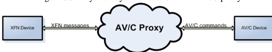
Figure 6.3: Physical layout of network with AV/C proxy
