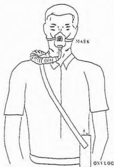
FIGURE 2: Attachment and positioning of the oxylog on a subject prior to testing.
