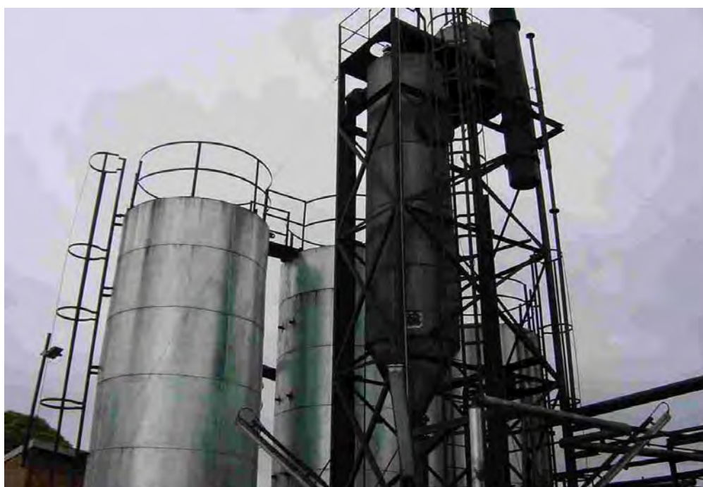
Figure 5.1 Water stripped off waste oils at FFS Refiners (Pty) Ltd. in the evaporator prior to cracking and recycling as furnace oils.
