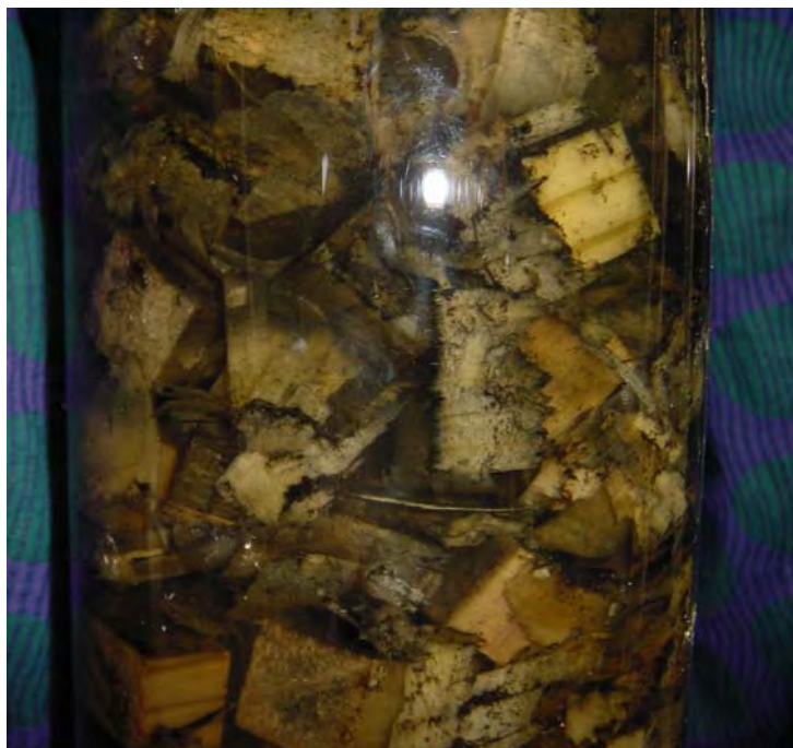
Figure 3.13 Black metal precipitates on the surfaces of wood chips due to sulphate reduction in the reactor.
