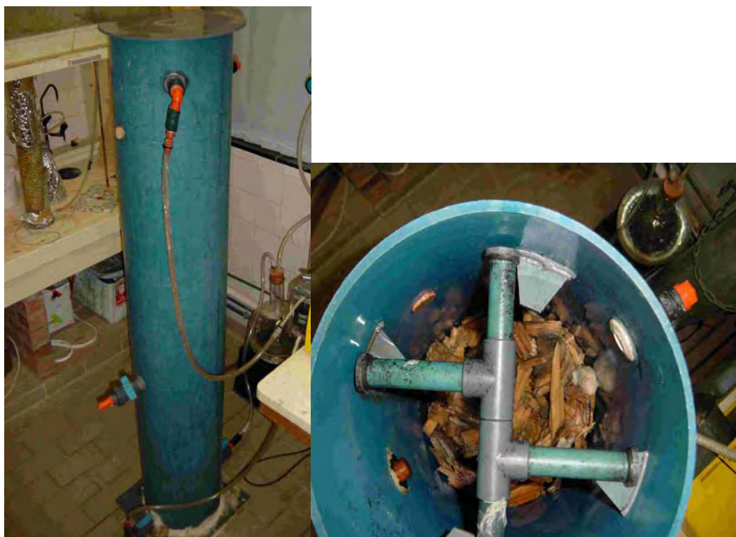
Figure 5.2 0.123 \text{ m}^3 trickling packed-bed reactor operated in the laboratory. Picture on the right shows the wood chip packing.
