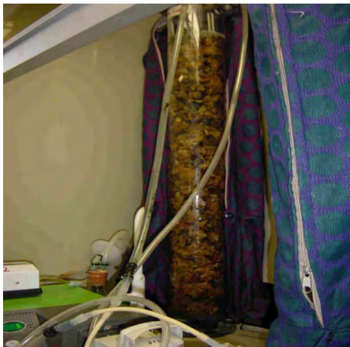
Figure 2.2 The pinewood chip-packed reactor operated in the laboratory.
