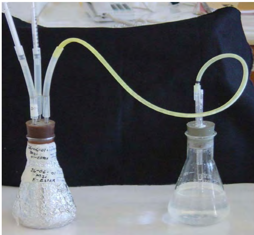
Figure 4.1: Batch reactor (left) connected to a zinc acetate sulphide trap (right) used to study the biodegradation of lignin and lignin model compounds. Flasks were covered with foil to prevent photosynthetic growth.
