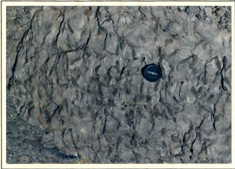
Plate 3.1 Spotted schists consisting of cordierite-biotite nodules within the foliation of the schist. The nodules occur within the schistosity but exhibit a decussate texture on the foliation plane.
