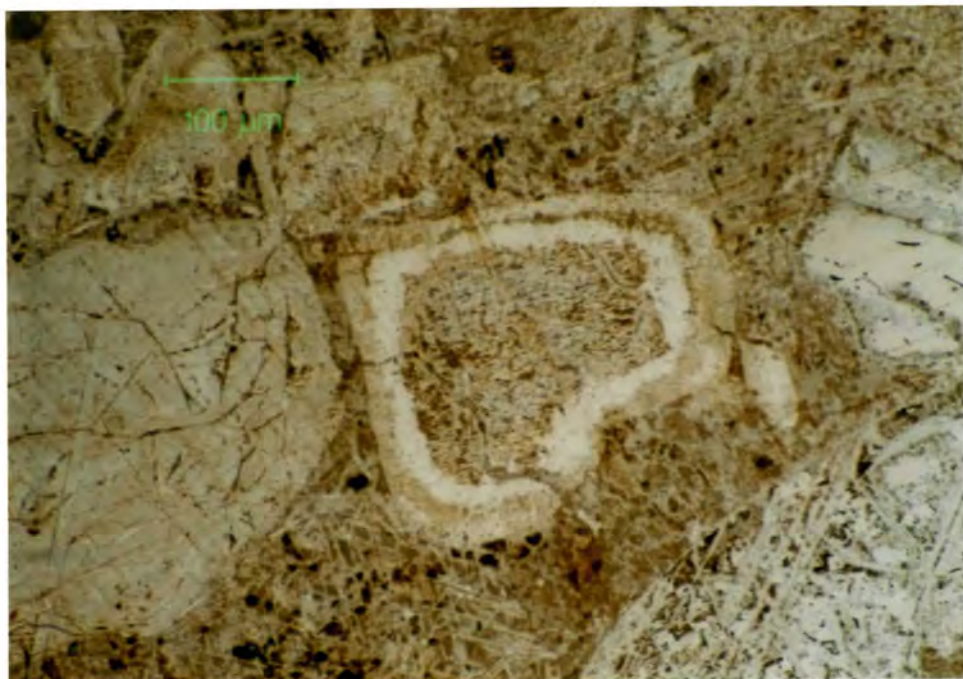
Plate 8. An altered ilmenite - leached ilmenite (LI) with a leached pseudorutile (LPR) centre, and a leucoxene (L) mantle. Reflected light, plane polarised.
