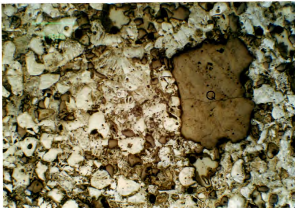
Plate 3. Plate shows the relatively poorly sorted nature of the grains. The large quartz grain (Q) is nearly 3mm along its long axis. Reflected light, plane polarised.
