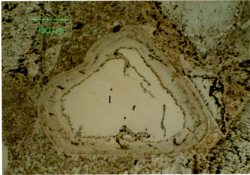
Plate 7. Ilmenite (I) within an alteration corona, which shows alteration from leached ilmenite to leucoxene (L). The leucoxene occurs as a very thin mantle. Reflected light, plane polarised.
