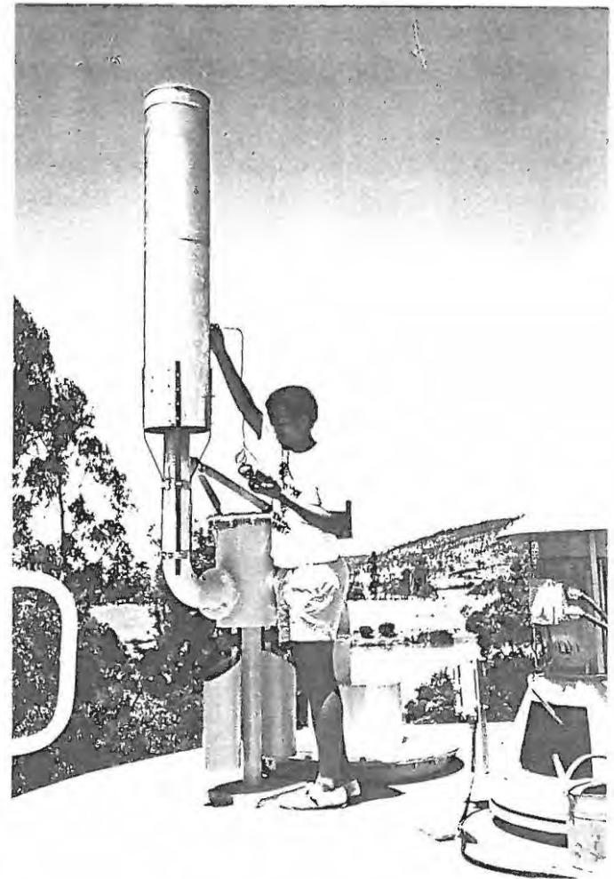
Photograph 2. Monitoring Biogas Flow Rates.
