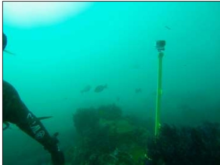
Fig 4.4 Go-Pro steel frame with weighted base standing 1m off the sea bottom.
