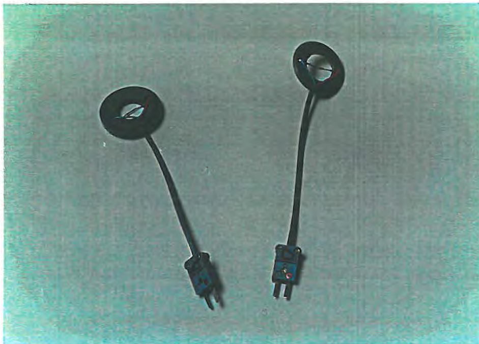
Figure 18 : Skin temperature sensors
