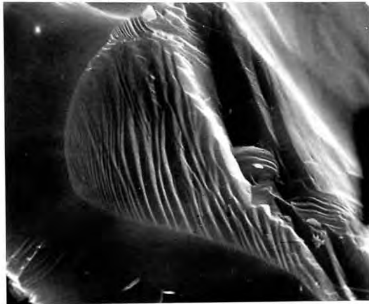
Fig.51: Ridge like forms observed on quartz grains (3000*; sample K-116)
