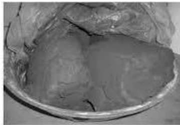
Fig.3. Wedged clay ready for use. (2007), photograph by Dr John Steele. (Available at: https://repository.up.ac.za/bitstream/handle/2263/10388/Steele_Rural(2007).pdf (Accessed: 31/01/2024)).
