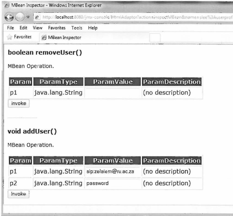
Figure A.5: The Mobicents XDMS web interface for creating and removing XDMS profiles
