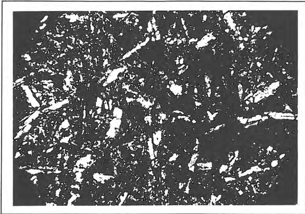
Plate 1.1.1 Photomicrograph of remnant basaltic lava. FOV = 1 mm
