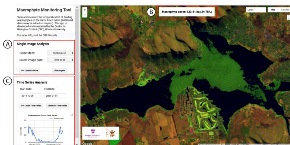
Figure 3.19: A screenshot of the WebApp built in GEE. A) Shows the options for a single image analysis. B) The map window that displays the selected image, with a cover estimate in both hectares and a percent. C) The time-series section, where users can request cover and NDVI time-series between specific data.
