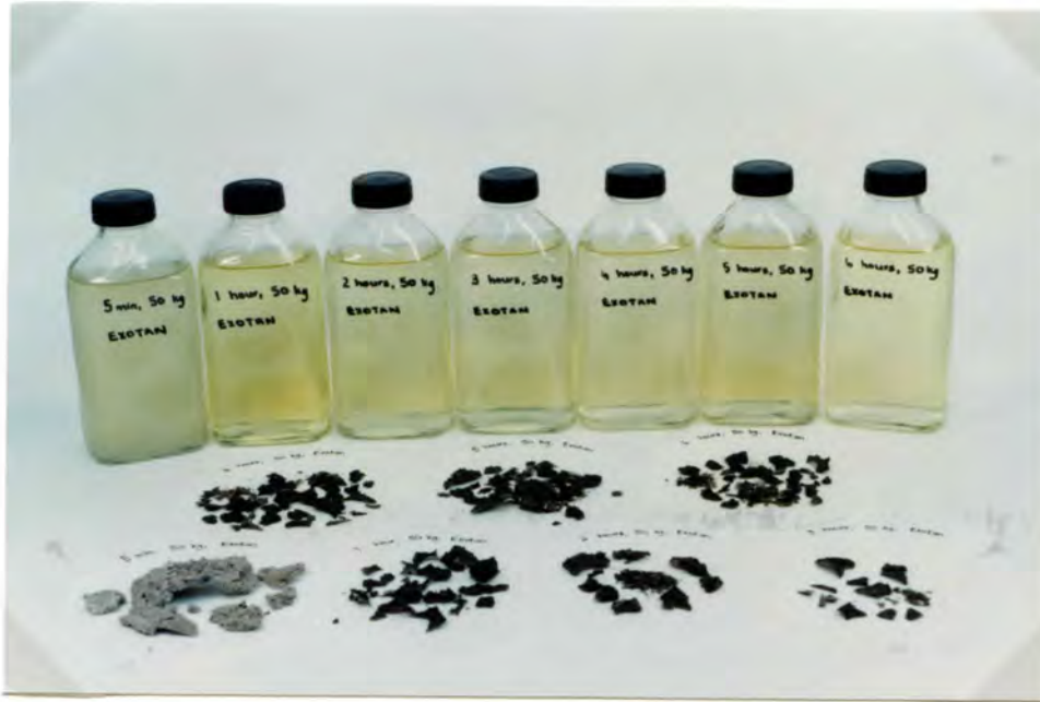
Plate 5.1. Alkaline hydrolysis filtrates and desiccated solid residues of the 50kg loading study.
