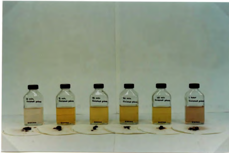
Plate 5.6a. Acid wash supernatants and solid residues (0 minutes–1 hour) of the finished leather trimmings.
