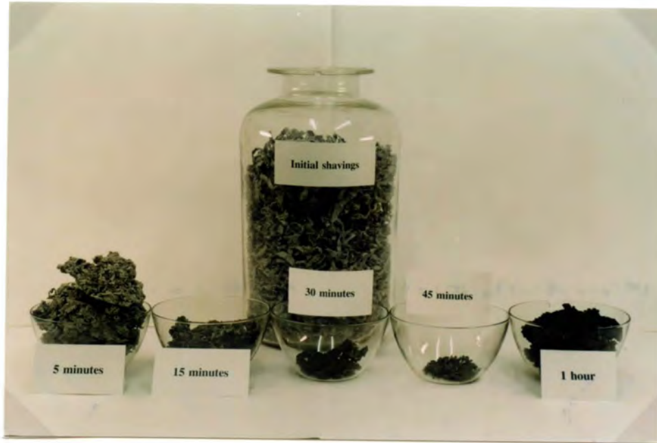
Plate 5.4a. Desiccated solid residues (5 minutes–1 hour) retained during size reduction analysis of the 220kg loading study.
