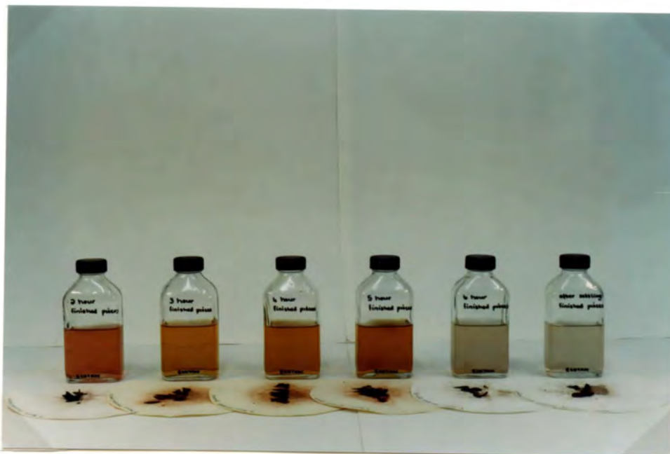
Plate 5.6b. Acid wash supernatants and solid residues (2–6 hours) of the finished leather trimmings.
