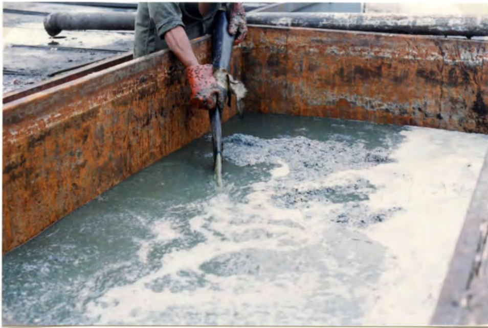
Plate 2.3. Introduction of the effluent to the reaction vessel prior to hydrolysis.
