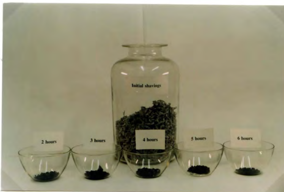
Plate 5.3b. Desiccated solid residues (2–6 hours) retained during size reduction analysis of the 100kg loading study.
