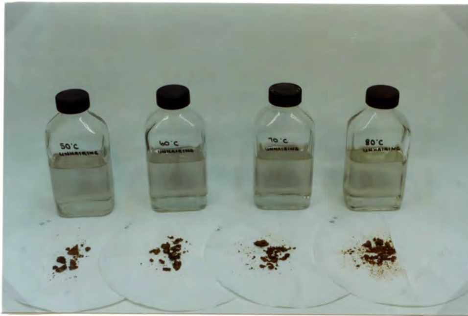
Plate 4.3. Acid wash supernatants and solid residues of the 50–80°C unhairing effluent samples.
