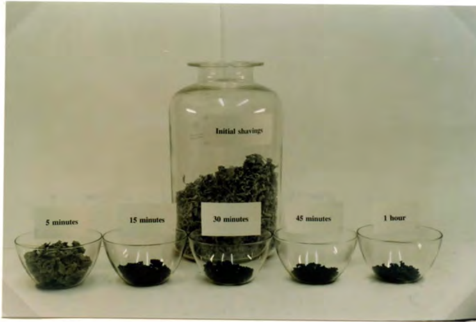
Plate 5.3a. Desiccated solid residues (5 minutes–1 hour) retained during size reduction analysis of the 100kg loading study.
