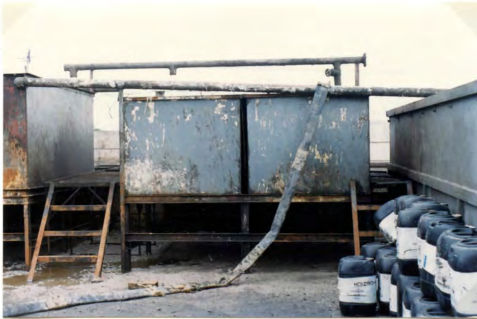
Plate 2.1. Reaction vessel utilised for hydrolysis of the solid wastes in the industrial-scale investigations.
